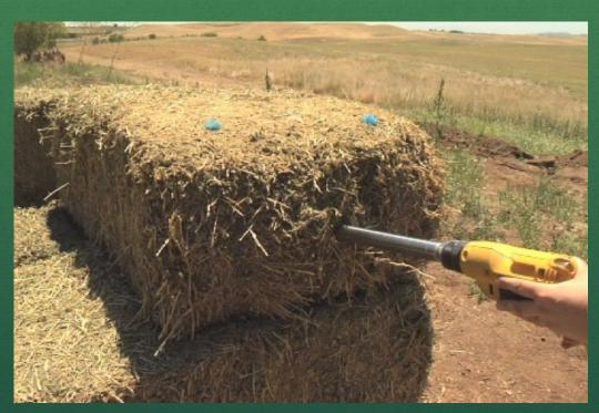
Insert corer into square bale, sample 20 bales, mix cores and seal in 1-gallon Ziploc bags.
